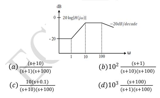
**Soln.** At  $\omega = 1$  change in slope 20 dB/decade Zero at  $\omega = 1$  $\omega = 10$ , change in slope 20dB to 0dB i.e. -20dB/decade pole at  $\omega = 10$  $\omega = 100$  change in slope -20dB/decade pole at  $\omega = 100$ Transfer function
