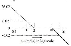
If the system is connected in a unity negative feedback configuration, the steady state error of the closed loop system, to a unit ramp input, is\_\_\_\_\_.
