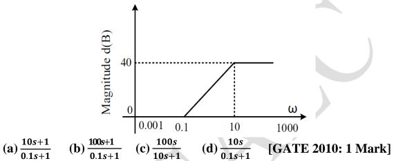
**Soln.** Slope of asymptote changes from 0 to 40 dB in 2 decades (0.1 to 1, 1 to 10) or slope is 20dB/decade
